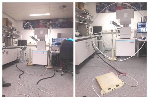
Figure 4: Test setup at SEM Left - Loop orientation for perpendicular field application Right - Loop orientation for parallel field application
