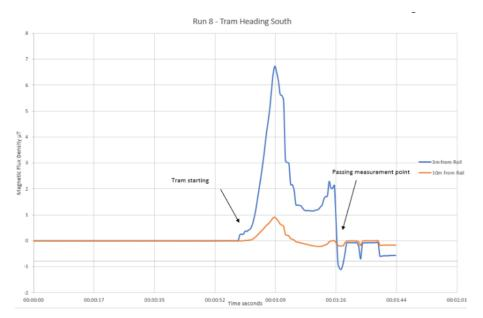
Figure 3: Magnetic flux profile of Luas passing measuring point at 3 m and 10 m distance
