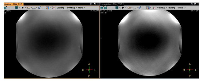
Figure 8: Baseline scan of test artefact (right) versus scan with varying DC field applied
